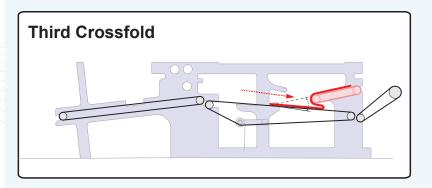
Finally, depending on item size and thickness, a **third crossfold** can be made by a combination of lifting guides and an inverter-driven reversing conveyor that raises and lowers to automatically compensate for thicker blankets, many types of bedspreads, as well as thinner items such as sheets.
