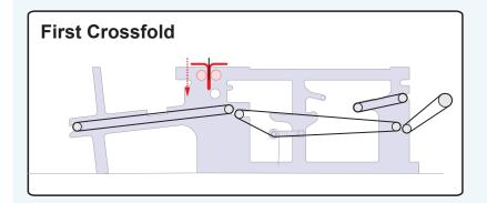
The **first crossfold** is performed by an oversized blade assembly pushing the primary folded item through pinch rolls with timed air pulse assist to prevent blankets from wrapping around rolls. Independent inverter-driven first crossfold runs only when needed for less wear and to ensure precision item positioning for crossfolds.
