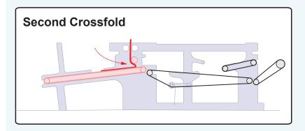
For improved accuracy and dependability, the **second crossfold** is performed by a clutch-free, inverter-driven reversing conveyor. The entire crossfold section is designed for open and direct access by maintenance personnel to keep production high and interruptions low.
