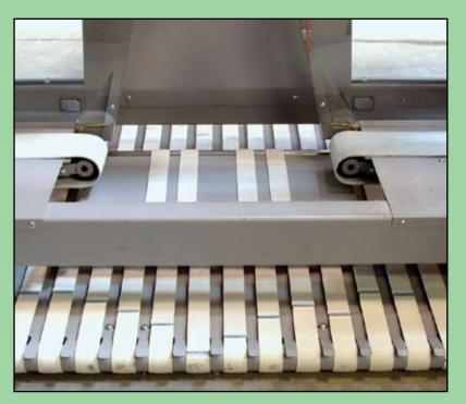
Bottom conveyor helps advance linen into the machine during feeding, while narrow reject conveyor automatically brings misfed pieces back to the front center and out of the machine to limit operator feeding interruptions.
