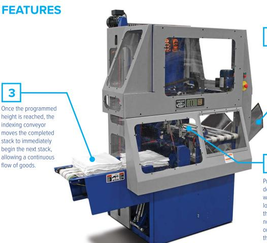
ATM<sup>2</sup> is automatically fed with tumble dried washcloths or other items of similar size funneled directly to a central hopper container from an overhead sling, conveyor, or cart. The items are gently pushed under a picking head at timed intervals where they are individually lifted from the hopper and properly oriented for stacking.
