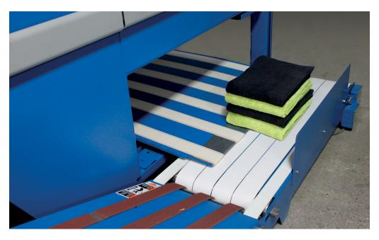
We covered all the bases with our newly redesigned Air Chicago Elite conveyor system. It is now possible for on-site reconfiguration of the discharge conveyor to a standard left/right discharge, return to operator, or to a master take away conveyor. Its new retractable gentle touch transition system ensures smooth operation and more accurate stacks, all while maintaining stack integrity throughout transition and delivery.
