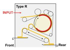
**Rear Return** allows flexibility, and increased production as additional piece processing is performed by separate receiving operators or a Skyline automatic folder
