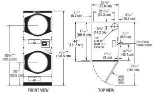
\*Dimensions will vary according to adjustment of leveling legs; add  $\frac{1}{2}$ " (1.3 cm) minimum.
