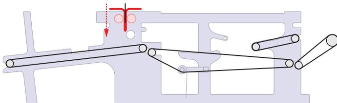
The **first crossfold** is performed by an oversized blade assembly pushing the primary folded item through pinch rolls with timed air pulse assist to prevent blankets from wrapping around rolls. Independent inverter-driven first crossfold runs only when needed for less wear and to ensure precision item positioning for crossfolds.
