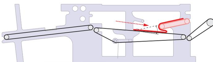
Finally, depending on item size and thickness, a **third crossfold** can be made by a combination of lifting guides and an inverter-driven reversing conveyor that raises and lowers to automatically compensate for thicker blankets, many types of bedspreads, as well as thinner items such as sheets.
