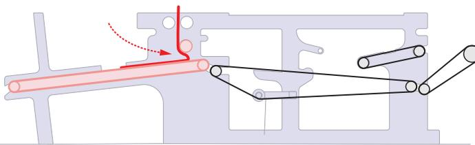
For improved accuracy and dependability, the **second crossfold** is performed by a clutch-free, inverter-driven reversing conveyor. The entire crossfold section is designed for open and direct access by maintenance personnel to keep production high and interruptions low.
