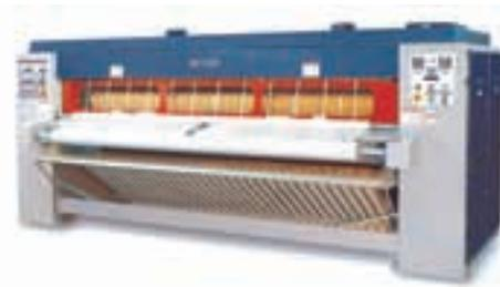
**Choice of 4 roll diameters and 2 heat sources and multiple roll widths to suit the needs of a wide variety of users.**
