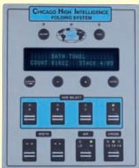
**CHI** is the first finishing control that successfully integrates the power of an advanced microprocessor with a message display and operator panel that anyone can easily use. During installation, a library of factory-programmed item descriptions is used to set up the correct number and style of folds for each item type to be processed. **CHI** stores all folding variables, including air pulse patterns,
